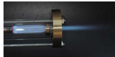
Figure 2, Transparent Hot Oxygen Device
