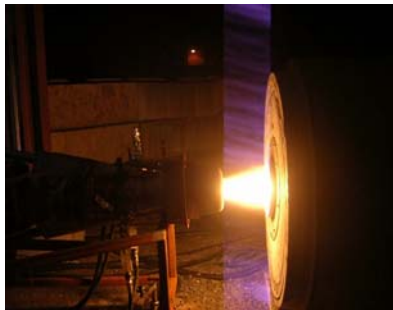
Figure 9, Combustion zone in hot oxygen mode
