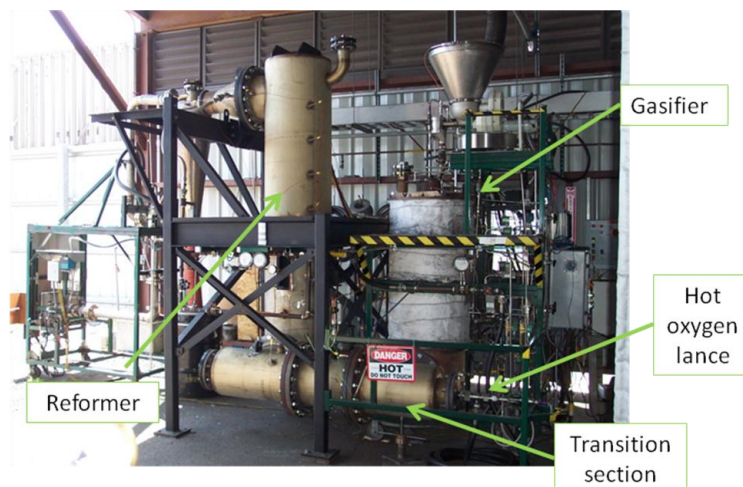
Figure 2. 1 ton/d entrained flow gasifier and reformer
