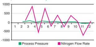
A typical autoclave cycle might involve several pressure and nitrogen flow changes during the curing process. Analyzing these patterns for single or multiple autoclave facilities is a critical step to providing the optimum nitrogen supply equipment and the design of the nitrogen distribution piping that result in reproducible results.
